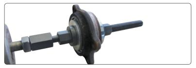
New principle for the screwed wheel bearings. Fits nearly all other wheel bearings as well. Makes it a solid connection, easier to remove when using slide hammer.
