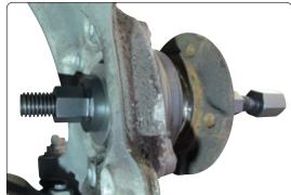
The master suspension kit can help you remove all components of the wheel knuckle. From the wheel bearing assembly, to the drive shaft push out and even lower ball joint/suspension arm removal.
