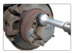
Special grinder used to clean the wheel rim contact surface, designed for vehicles with stud bolts. Corrosion is quickly and easily removed.
