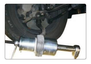
Sleeves outer diameter from: 44 - 82 mm
