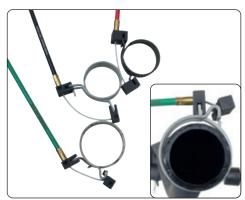
The automobile manufacturers increasingly rely on hose clamps with tight-fitting jaws, which are difficult to open with conventional tools and hard to reach in very narrow areas.
