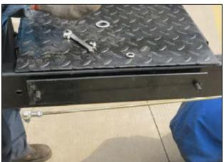
16. Route and mount the appropriate Cable(s) (Items # 94, 95, 96 & 97) to each Column Top Cap, while ensuring that the small, spring loaded Cable Pulley (Item # 41) is between the Cable and the Lock Ladder. This will allow the secondary slack cable lock to function properly. See Figure # 4 for Cable routing installation. **Note:** Make sure all Cables are properly routed around Cable Sheaves.
