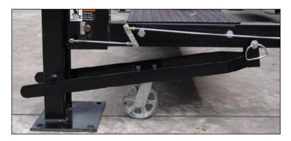
4. Lower lift and the columns will automatically raise off the floor.
