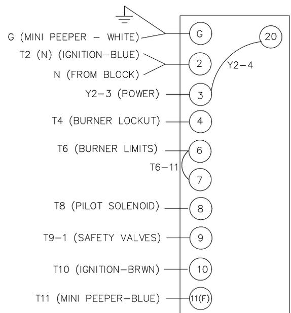
The flame controller is responsible for flame safety but it does not control the intensity of the flame. After the burner is ignited, the PLC starts regulating the spray booth temperature. Through the mod valve, the PLC increases or decreases the fuel supply to the burner to create more heat or to create less heat.
