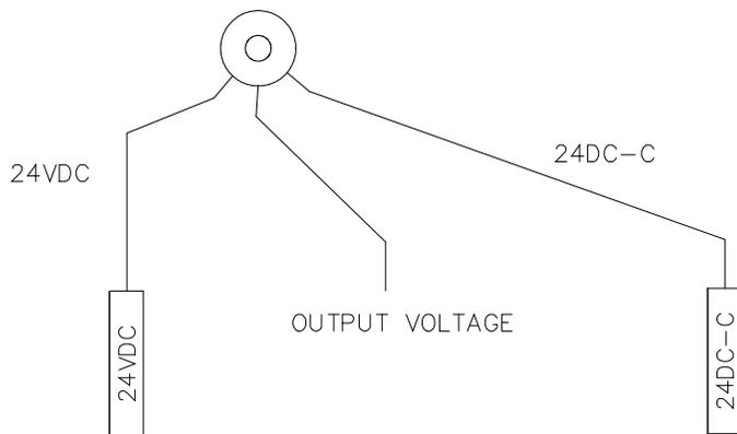
Measure DC on the center terminal while turning the potentiometer L to R.
