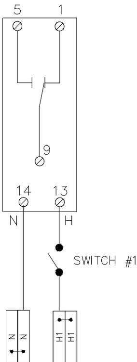
3. Wire the red light to 5 and a green light to 1. Turn the relay on and off.
