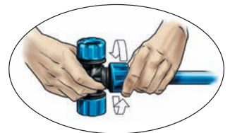
4 - Tighten nut 1/2 turn past "hand tight" with wrench
