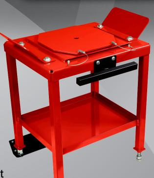
This design in wheel alignment stands has the Turnplates and slip plates built right into the stands. These stands are made with 1/4" steel tops and are rated at 2500 lb. per stand.
