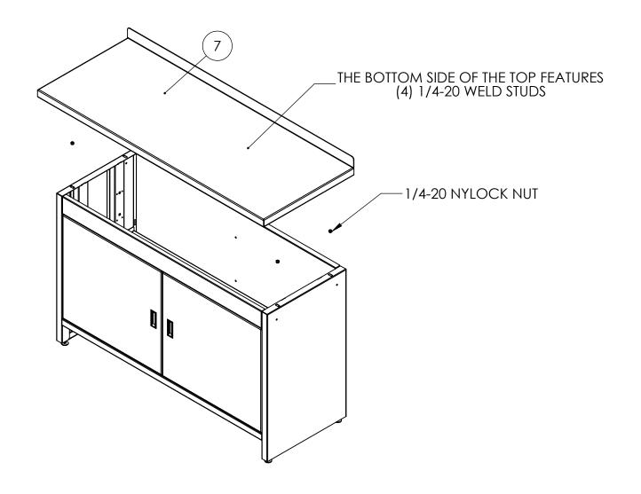
INSTALL WORK TOP USING (4) NYLOCK NUTS FROM INSIDE CABINET. ENSURE ALL FASTENERS ARE TIGHTENED AND EVERYTHING IS SQUARE.
