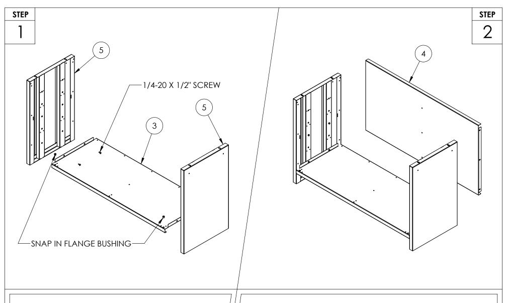
USING (4)  $1/4-20~\rm X~1/2"$  SCREWS, WITH THE LEFT & RIGHT PANELS STANDING UPRIGHT, INSTALL THE CABINET BASE.
