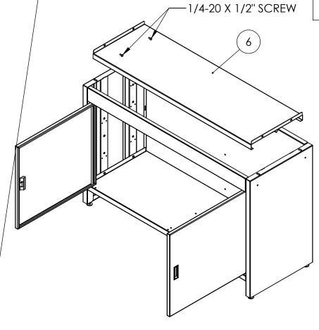
INSTALL DOOR HARDWARE INTOBOTH DOORS. PLACE DOORS THROUGH BOTTOM BUSHINGS, THEN LOWER UPPER PANEL INTO PLACE AND SECURE WITH **SCREWS & NUTS**
