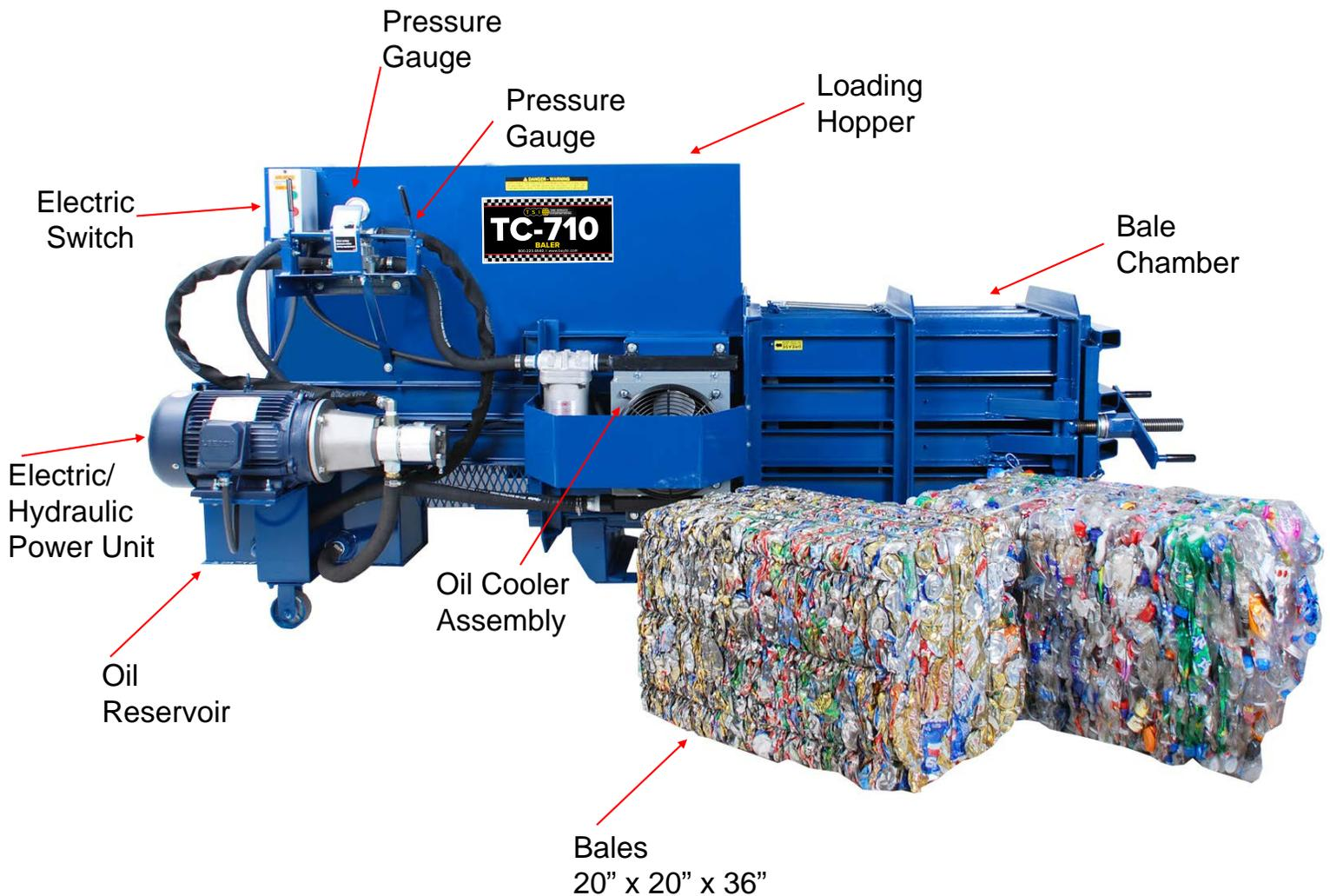
*NOTE:* Fig. 1 displays an electric unit. Gas units have the power source located on the opposite side of where electric motor is mounted.
