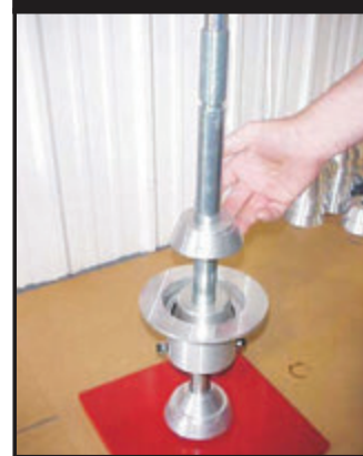
Step 9 Placing retaining unit over shaft (Hold out 2 knobs)
