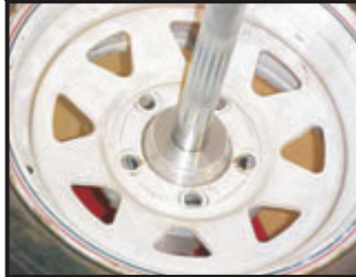
View 1 Unlocked position to remove retaining unit
