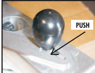
View 1 Unlocked position to remove retaining unit
