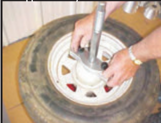
Step 10 Retaining unit in position, turn approximately ¼ turn to lock
